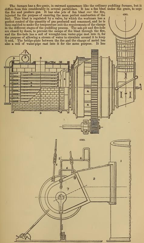
a lining of fire-brick on the side next to the fire, and a covering of fettling on the side next to the charge. It also has a course of fire-brick on the top, and is thus perfectly protected on all sides. Fastened on to the bridge-plate is a 4363.
